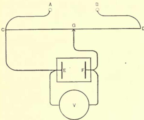
primary batteries, secondary batteries, dynamo or lightning circuit. The electrolytic cell is connected so that one pole E connects with C and the other pole F connects with the movable point or slider G so that any point of the conductor CD can be selected and any voltage from zero (when G is at C) to the full
